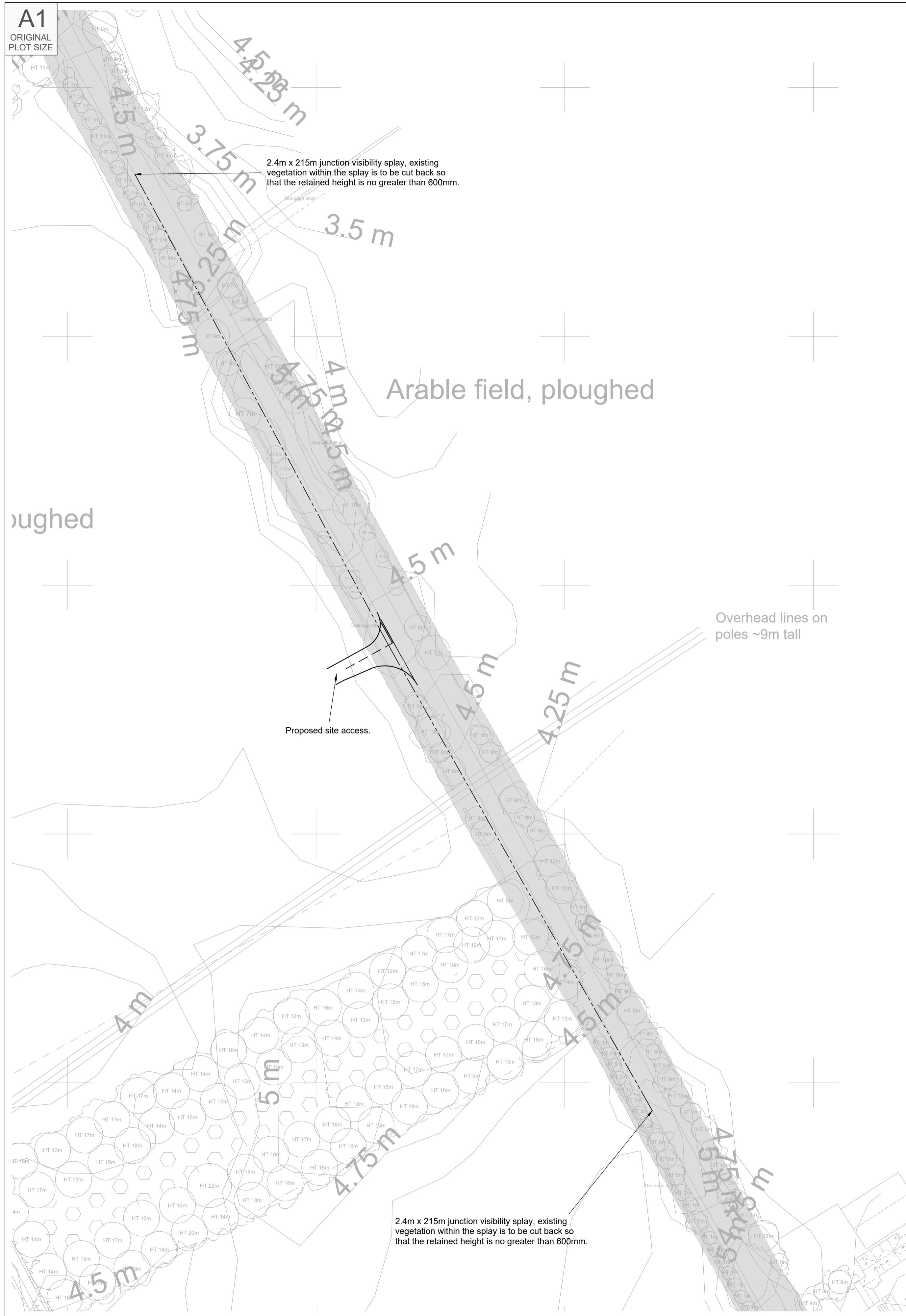
Site Access Arrangement and Visibility Splays
